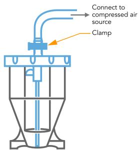
Figure 9 Connect Compressed Air
