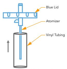
Figure 7 Assemble the Nebulizer
